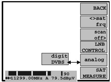
Press the button *sat frq* and enter the transponder frequency 11299 MHz with the numerical buttons. Confirm the entry with the MHz button. You will now see the frequency and level in the lower display field.
